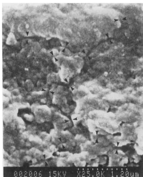
FIG. 6 SEM photomicrograph of the cross section of the top coated layer of SPPO polymer of the same TFC-SPPO membrane sample as shown in Figs. 4 and 5 at a higher magnification of 25,000\times .
