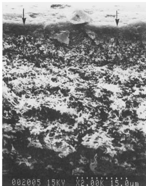
FIG. 4 Scanning electron microscope (SEM) photomicrograph of the cross section of a thin-film composite (TFC) charged SPPO ultrafiltration membrane.
